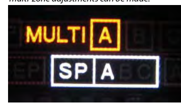
The 'MULTI (A)' indicator flashes when the SR5003 is in multi-zone mode. While flashing, multi-zone adjustments can be made.
