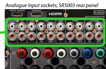
Analogue input sockets, SR5003 rear panel
